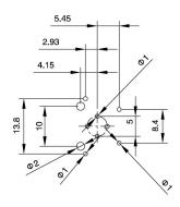
Recommended PCB thickness:1.6mm
