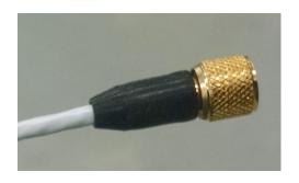
Crimp the barrel with 0.151 in HEX crimp die. Trim shield. Push boot over the rear barrel.
