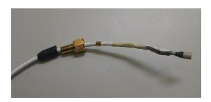
Trim the wires to 0.200 in and strip conductors to 0.05 in for soldering. Shrink thin wall tubing over the contacts. Tape the flattened shield to the cable.
