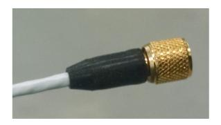
Crimp barrel with 0.151 Hex crimp die. Trim shield. Push boot over rear of barrel.
