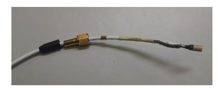
Trim the conductors to 0.225 " and solder the contacts. Shrink thin wall tubing over contacts. Tape the flattened shield to the cable jacket tape.
